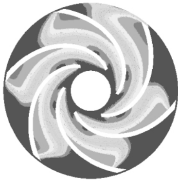
图 8 漩涡汽蚀阶段气相体积分数分布 Fig. 8 Distribution of gas phase volumetric fraction when a vortex-caused cavitation takes place
