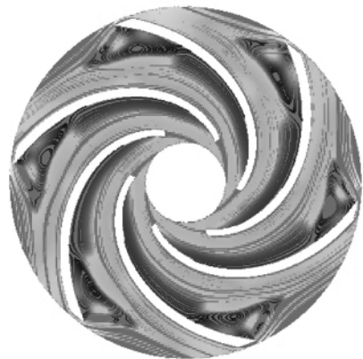
图 11 漩涡汽蚀阶段流线云图 Fig. 11 Cloud atlas streamlines when a vortex-caused cavitation takes place
