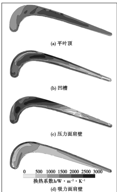
图 7 叶顶表面换热系数分布 Fig. 7 Heat transfer coefficient distribution on the tip surface
