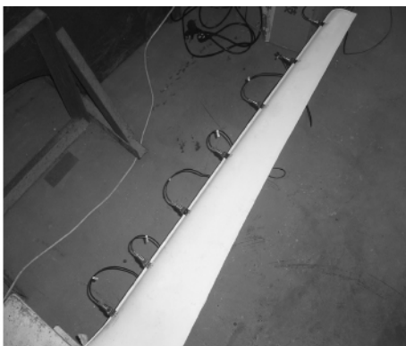
图 2 传感器横向布置测量摆振方向 Fig.2 Vibration along the flapping direction measured by the sensors arranged in the lateral direction
