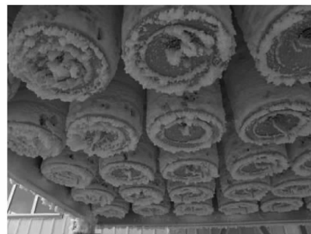
图2 塔里木盆地燃气轮机滤芯结冰实景 Fig. 2 Real conditions of the cartridge of a gas turbine iced in Tarim basin
