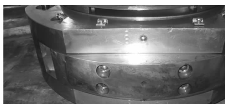
图3 1号轴承支撑垫块的球面示意图 Fig. 3 Schematic drawing of the spherical surface of a support pad of the bearing No. 1
