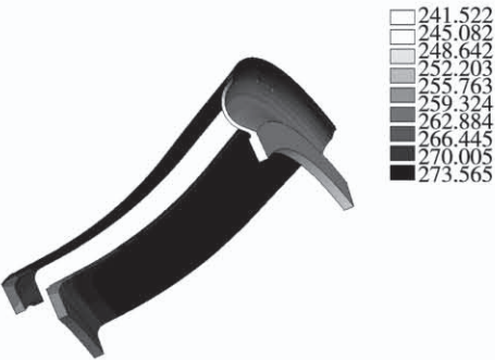
图 8 慢车工况下内罩壳与月牙板温度分布图(℃) Fig.8 Temperature distribution of low speed condition of inner enclosure and crescent-shaped plane(℃)
