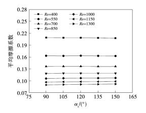
图 17  $\alpha_s$  对微通道平均摩擦系数的影响 Fig. 17 Effect of  $\alpha_s$  on average friction coefficient of microchannels
