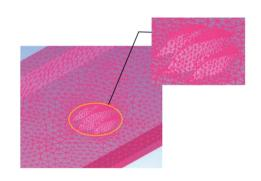
图 2 仿生鳞片结构微通道局部网格划分示意图 Fig. 2 Schematic diagram of local grid division of microchannels of biomimetic scale structure
