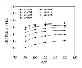
图 19  $\alpha_s$  对微通道综合性能因子的影响 Fig. 19 Effect of  $\alpha_s$  on comprehensive performance factor of microchannels
