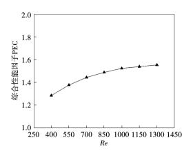
图 8 鱼鳞结构微通道综合性能因子随雷诺数变化 Fig. 8 Variation of comprehensive performance factor of fish-scale microchannel with Reynolds number
