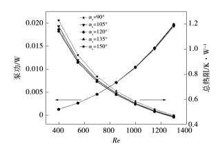
图 20  $\alpha_s$ 对总热阻和泵功的影响 Fig. 20 Effect of  $\alpha_s$  on total thermal resistance and pumping power
