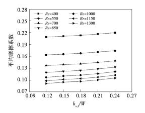
图 9  $b_{s,1}/W$  对微通道平均摩擦系数的影响 Fig. 9 Effect of  $b_{s,1}/W$  on average friction coefficient of microchannels
