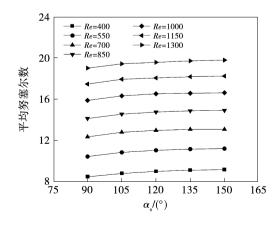
图 18  $\alpha_s$  对微通道平均努塞尔数的影响 Fig. 18 Effect of  $\alpha_s$  on average Nusselt number of microchannels
